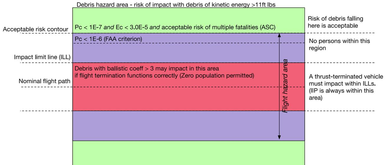
Figure 3-4 Flight hazard area and ILLs
