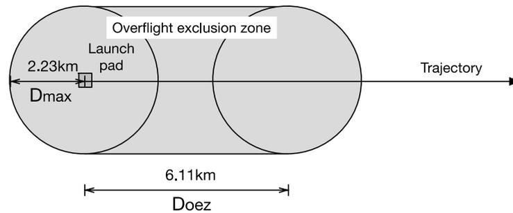
Figure 3-1 Overflight exclusion zone for small launch vehicle class
